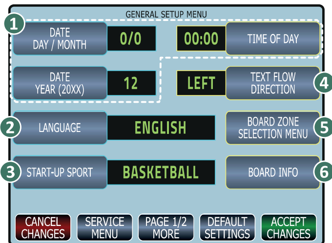
Fig. 2 – General setup menu, page 1/2. The bottom buttons are elaborated on the next page.
