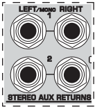
Fig. 2.8: Stereo aux return connectors
